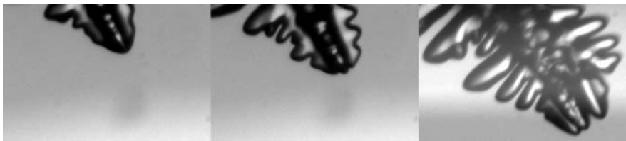
Fig. 3. A crystal with three tips is formed in a similar process as observed in Figure 1.
